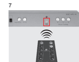
If necessary ; use I.R remote controller to fine tune R.G.B skew
